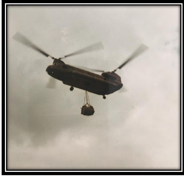
The primary means of delivering supplies to Fire Support Bases in Vietnam was by sling load. This was a load of “Class V” or Class Five”, which in military parlance is ammunition of all types including, bombs, explosives, mines, fuses, detonators, pyrotechnics, missiles, rockets, propellants, and associated items. Photo by Steve Wolak.
