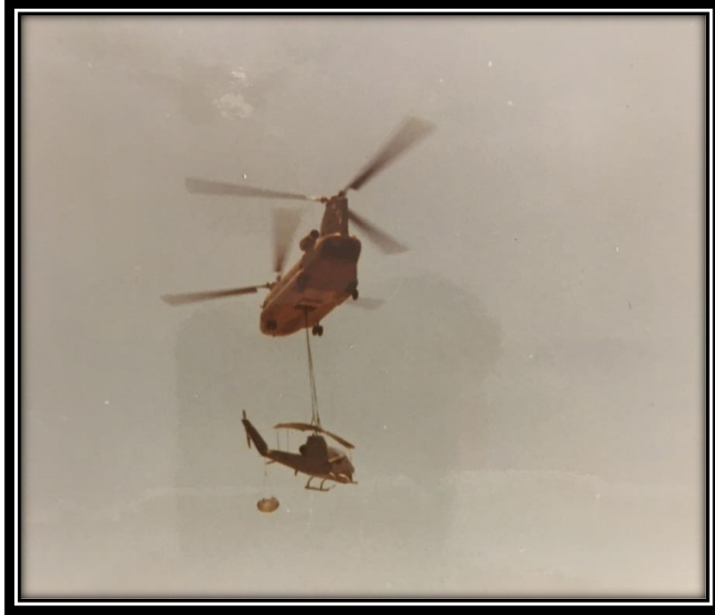
A Huey-cobra gunship sling-loaded beneath a CH-47. Note the drogue parachute to help align the gunship with the slip stream. If the external load starts uncontrollably spinning and if “pulling G’s” on the load (pulling up on the collective to increase the fuel flow into the helicopter’s jet engines and also increase the rotor blades’ angle of attack and “bite” in the air)...if this flight technique doesn’t reduce or stop the spinning, the load could be dangerous to the CH-47 and crew and might be jettisoned. It was enjoyable to unmercifully goad the “snake” pilots when one of their aircraft had to be saved by a heavy-lifter like the CH-47. Photo by Steve Wolak.
