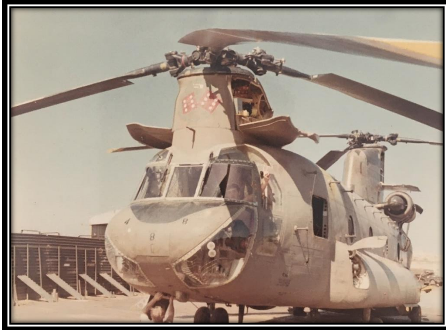
One of Steve's Assault Support Helicopter Company's "Box Car" CH-47's "unbuttoned" by the enlisted aircrew for preflight at Chu Lai. They'll "button it back up" prior to takeoff. Photo by Steve Wolak.
