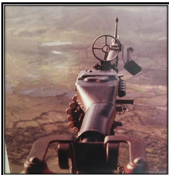
Steve's view from behind the "D" model M-60 (named as such because of the "D" shaped double handles on the weapon) in a CH-47 over Vietnam. Photo by Steve Wolak.
