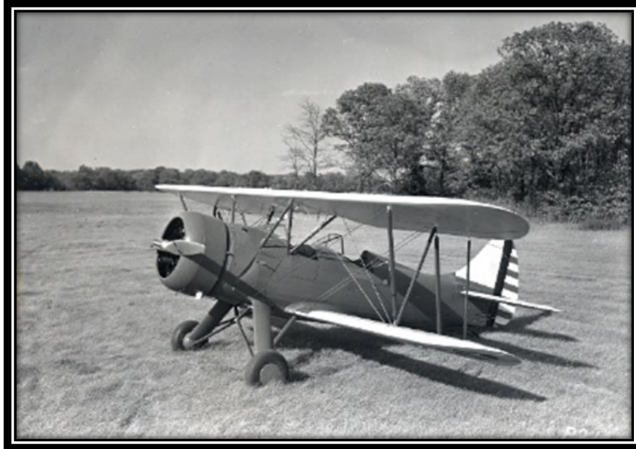
1939 WACO YPT-14A, with the Townend Ring installed, developed as a WWII trainer, which later became the civilian UPF-7. Photo courtesy the National WACO Club.
