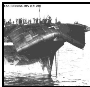
Severe bow damage on USS Bennington’s (CV-20) bow flight deck from the 1945 Okinawa Typhoon (Photo credit: US Navy)
